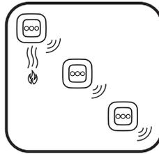
Each Sensor will act as a repeating station, so critical signals received by a Sensor will be rebroadcast throughout the network.
