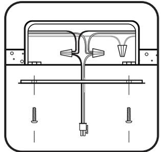
**With the AC power turned off**, connect the provided wire harness to your power lines. Using the orange wire nuts provided, connect the black wire of the harness to the black wire(s) in the electrical box, the white wire of the harness to the white wire(s) in the electrical box. Wire nut the red wires together or cap as shown.
